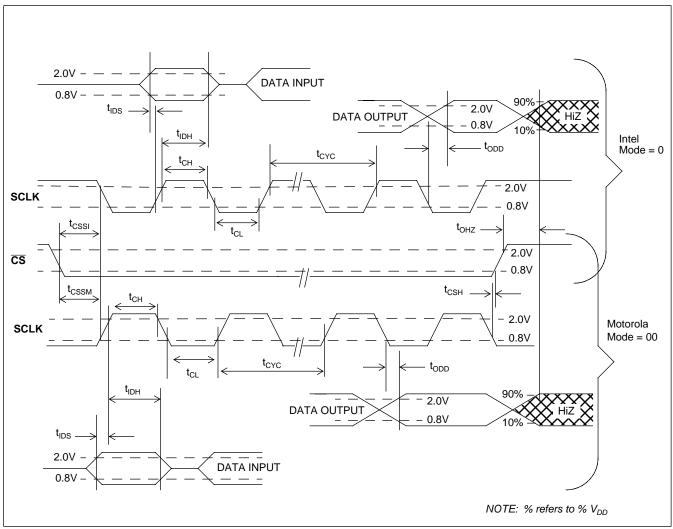
Figure 14 - Microport Timing
