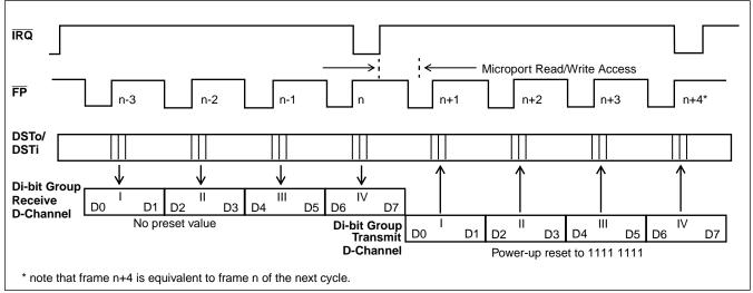
Figure 7a - D-Channel 16 kb/s Operation
