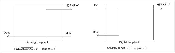
Figure 8 - Loopback Signal Flows
