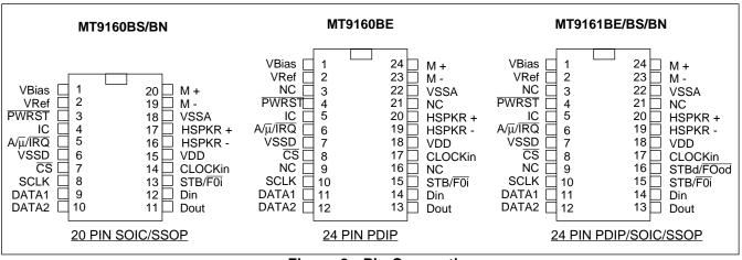
Figure 2 - Pin Connections
