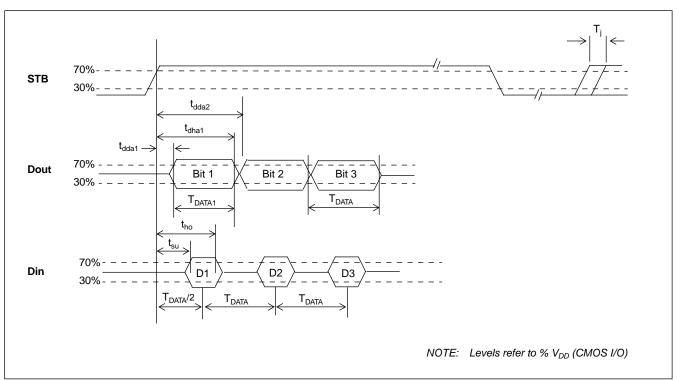
Figure 13 - SSI Asynchronous Timing Diagram
