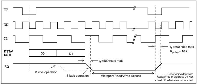
Figure 7b - IRQ Timing Diagram
