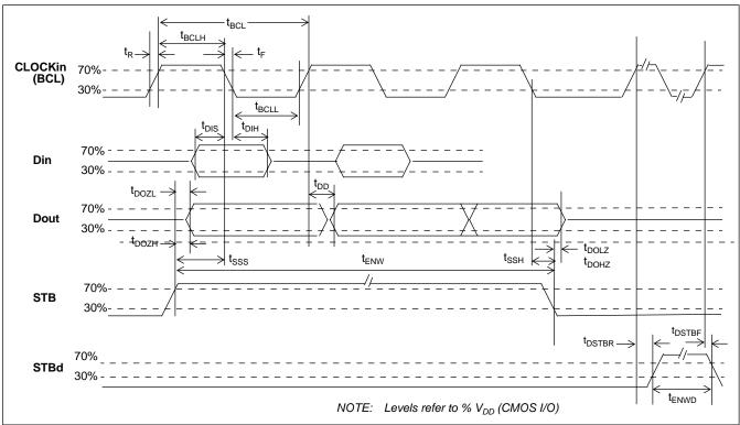
Figure 12 - SSI Synchronous Timing Diagram
