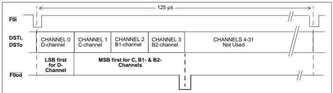
Figure 6 - ST-BUS Channel Assignment
