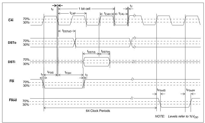
Figure 11 - ST-BUS Timing Diagram
